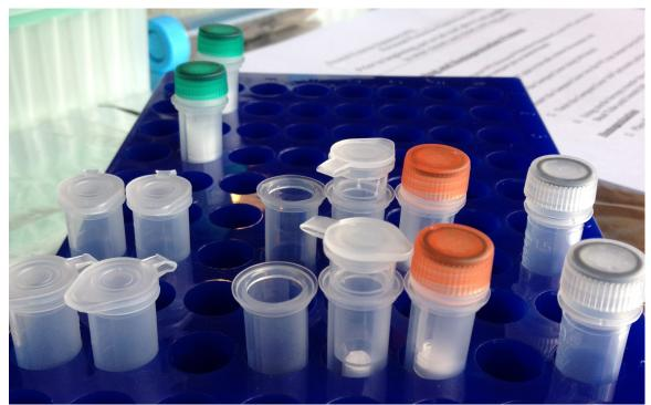
(<u>Tubes per sample extraction</u>: 4 Collection Tubes, 1 **BEAD** Tube, 1 **ORANGE** Filter, 1 **GREEN** Filter, 1 **WHITE** Filter, 2 Microcentrifuge Tubes)
