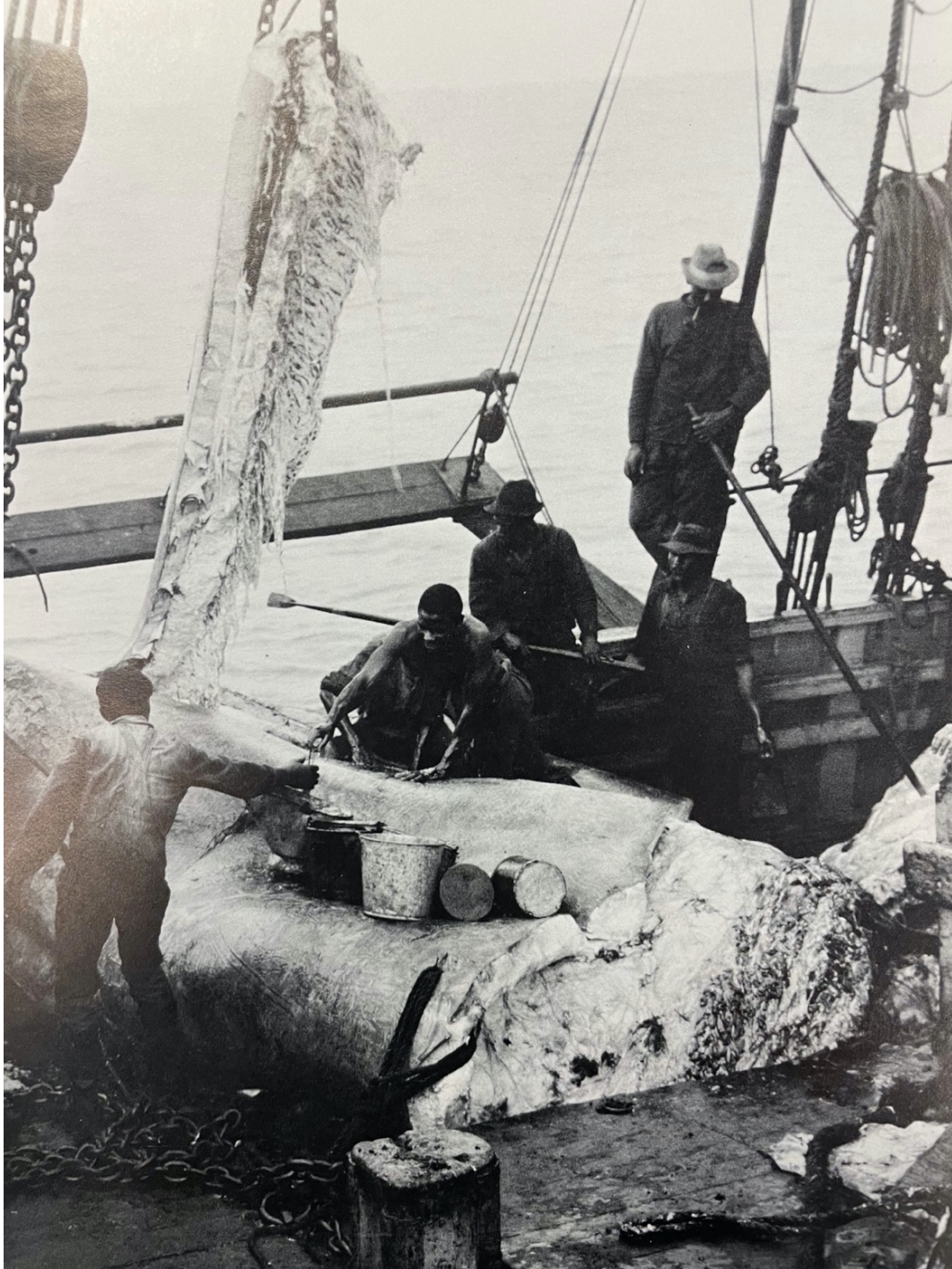
The American fishery perfected the spiral method of cutting in, aided by the heave of the windlass, roiling the whale in the water and excising blubber in continuous strips. Whale bodies were dissected and dissociated with increased speed/efficiency.
