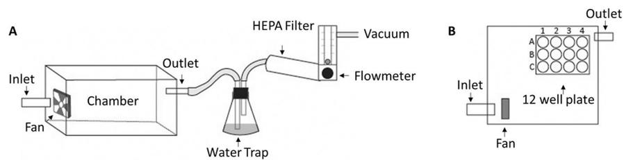
**Figure 1.** Experimental setup: (A) Exposure system for e-cig generated aerosol and (B) top view of the exposure chamber with placement of the transwell plate used for chemical characterization or in vitro exposures.
