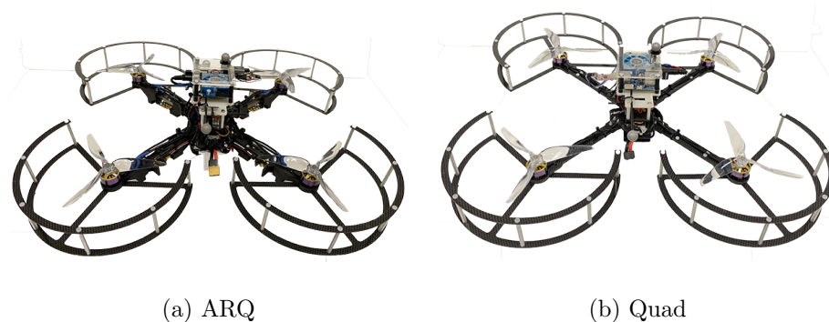
Figure 2.8: Our prototype of compliant (a) and rigid (b) robots. The robots share almost the same configuration except for their arms. Both robots measure 0.60 m from the cage tip to tip and 0.38 m from the motor tip to tip.
