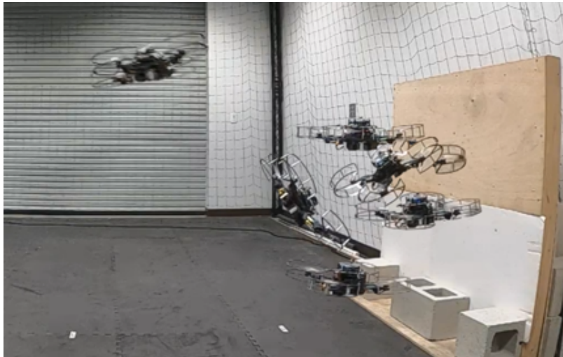
Figure 2.1: The compliant MAV developed in this work can rapidly stabilize from collisions with vertical walls at speeds of up to 3.5 m/s and sustain post-impact flight by tracking aggressive recovery trajectories. Composite images are made with a camera in 240 fps.
