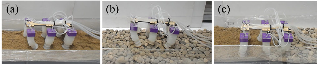
Figure 5.12: SoRX was found capable to traverse (a) sand, (b) rocks, and (c) mixed terrain.
