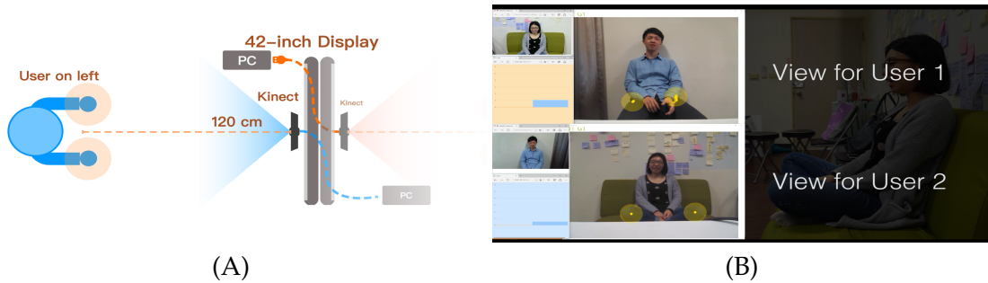
Figure 5.1: Overview of the HandVis video conferencing system used in the study: (A) physical configuration of the video setting [164]; (B) user interfaces seen by both users of a video chat [163]
