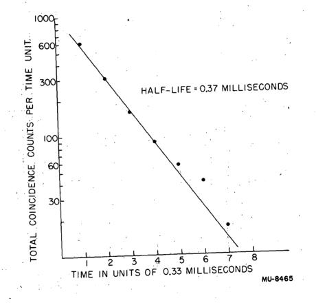
Fig. 2. Decay curve for Y<sup>88m</sup>. Data compiled from 17 photographs as described in text.
