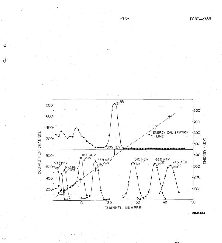
Fig. 1. Gamma spectrum of pure sample of Zr<sup>88</sup>.
