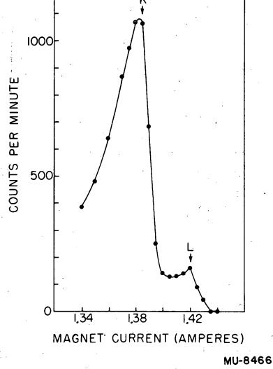
Fig. 3. Conversion electrons of 395-kev transition in Y<sup>88m</sup>. Data taken by O'Kelley.
