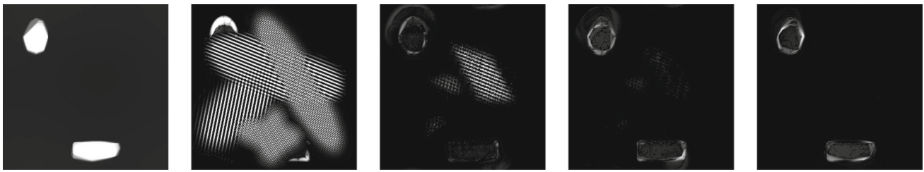
Fig. 3 Synthetic overlapping texture: 2D Prony–Huang decomposition (default parameters) [60]. Decomposition into trend and 4 modes; spectral analysis not shown
