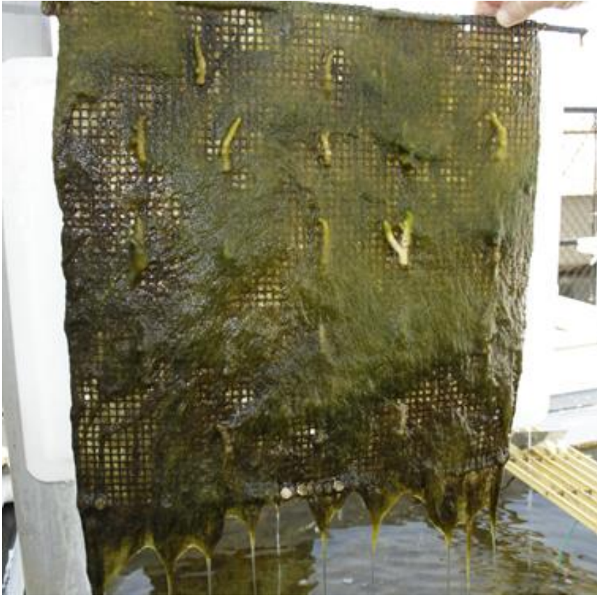
Figure 20. Plastic screen from Unpowered tank on Day 56 with smothered corals.
