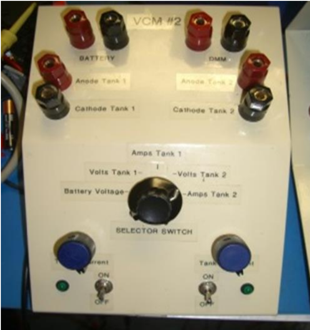
Figure 5. One of the dual-output Voltage Control Modules (VCMs) built for the project.
