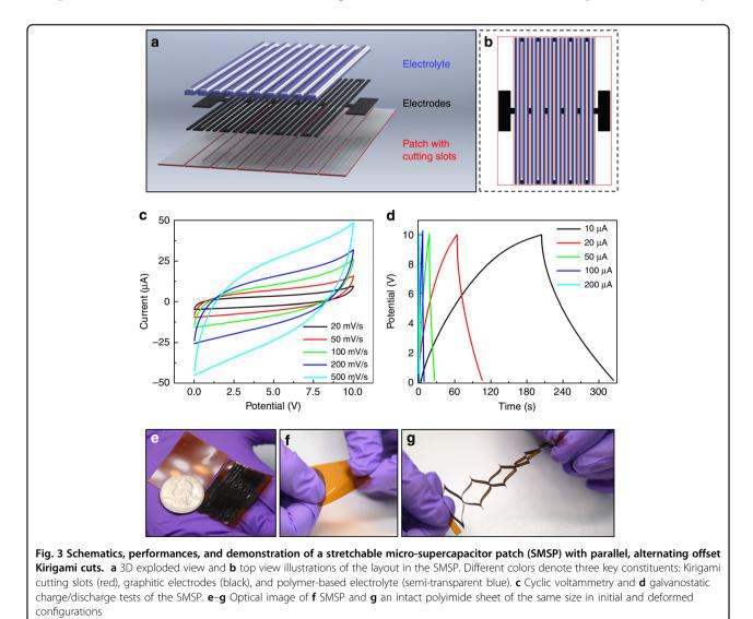
mm, which is only slightly larger than a US quarter (Fig. 3e). The pre-designed alternating, offset Kirigami cuts transforms the polyimide sheet into five deformable units that are mechanically (and electrically) joined together. Each deformable unit consists of two equivalent parallel plate-like capacitors joined in series. In total, the SMSP has ten equivalent capacitors of the same design in series connection.
