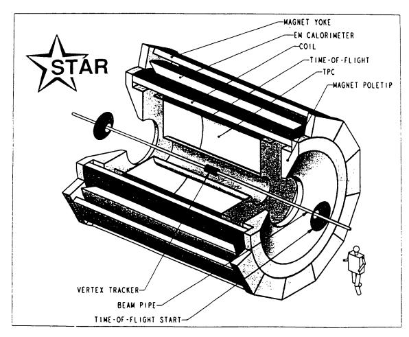
Fig. 1. Conceptual layout of the experiment, with cylindrical symmetry around the beam axis. See text for description.
