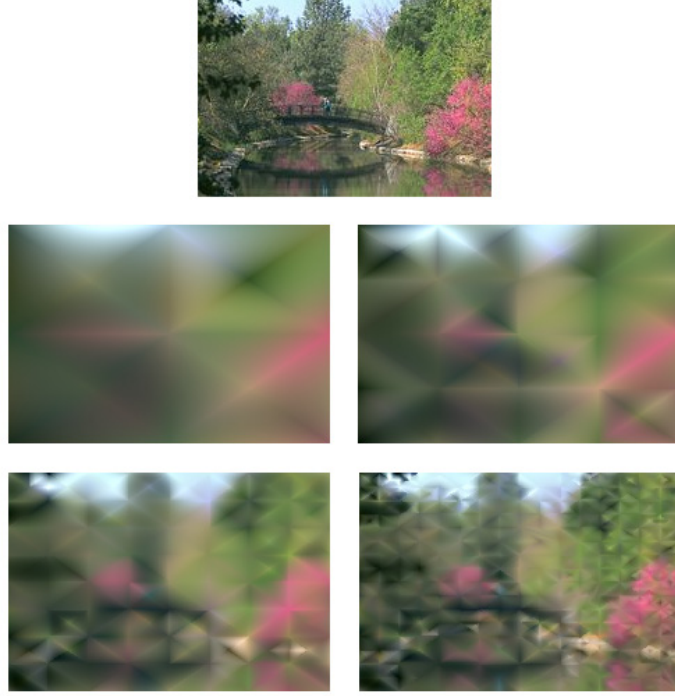
Figure 3.7: Quadratic hierarchical approximation of digital image data set. Original image is shown at the top. Four approximations are shown, from upper-left to lower-right, using 16, 48, 191, and 790 quadratic elements, respectively.
