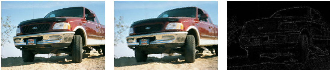
Figure B.2: Image-space error measurement. Left image shows the original. Middle image shows the approximation. Right image shows the difference image (error E being 3.56%).
