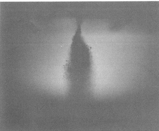
Fig. 7(b) Effect of liquid properties on "cellular breakup": side view, water and ethanol (Case 26)
