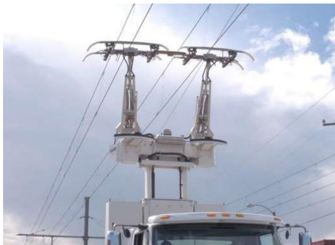
Figure 7. The eHighway pantograph. It is used to transfer the energy from the overhead lines to the electric motor on the truck [47].
