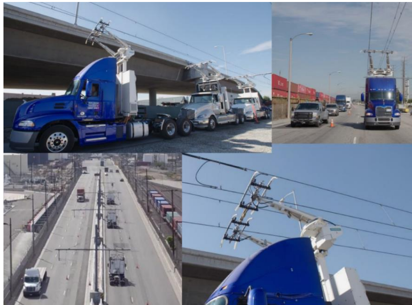
Figure 10. Alameda Street eHighway pilot project. (Top left) shows the three trucks adapted to run on the eHighway system, (top right) shows one of the trucks driving along with the system next to regular traffic, (bottom left) shows an aerial view of the catenary system, and (bottom right) highlights the pantograph engaged with the catenary [51].
