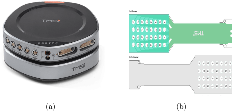
Figure 3.1: Hardware components of the experiments. a) TMSi SAGA 32+/64+ High Density Amplifier. b) TMSi 4-8-L HD-EMG Electrode layout. The EMG activity that occurs during typing is detected via the TMSi 4-8-L HD-EMG Electrodes, which have 32 channels equally spaced out. The detected signals are then collected by the TMSi SAGA 32+/64+ High Density Amplifier.
