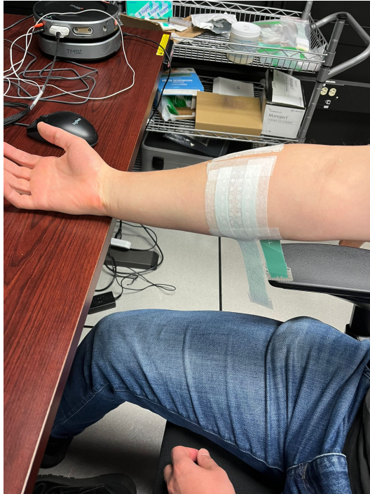
Figure 4.5: Alternative placement of the electrodes. To determine the effect of electrode orientation, the alignment of the electrodes was changed to be perpendicular to the anterior superficial muscles of the forearm in a horizontal position. To minimize movement artifacts, the electrodes were secured in place with adhesive tape.
