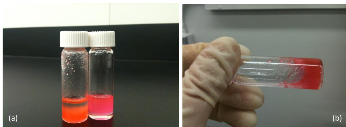
Figure 2.2: (a) Sample after ultrasonication (Left) and before sonication (Right); (b) Status of Sample (0.6g NaI dissolves in aqueous phase) after sonication
