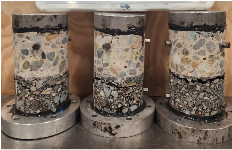
Figure 5.6: Composite specimens after UTM-ramp testing (PLCC on HMA).
