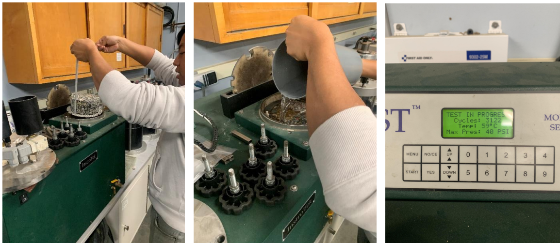
Figure 2.15: MiST device: specimens added to the chamber (left), chamber filled with water (center), and ongoing test (right).
