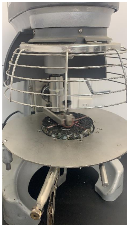
Figure 2.14: Erosion test on HMA.
