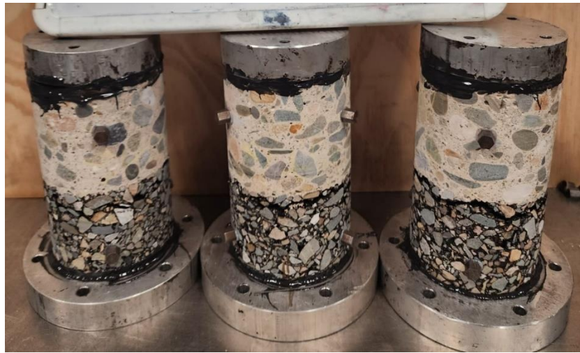
Figure 5.7: Composite specimens after UTM-ramp testing (PLCC on RHMA-G).
