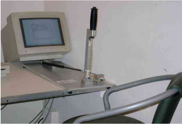
Figure 1. The response lever in the Away condition. The apparatus is rotated 180 degrees for the Toward condition.
