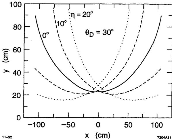
Figure 2: Loci of Cherenkov images from a  $\beta = 1$  track on a detection surface at 100 cm from the radiator bar end. Only the upper half of the image is shown. The images are shown for a dip angle  $\theta_D$  of  $30^\circ$  and three different azimuthal angles  $\eta$ .
