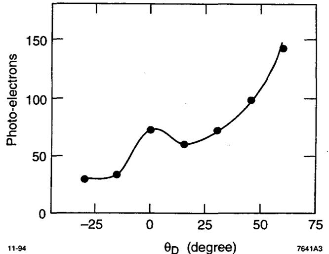
Figure 5: The observed photo-electron yield from a 1.7 cm thick bar at a track position  $z = 60$  cm as a function of dip angle  $\theta_D$ . The solid line is a Monte-Carlo simulation. The statistical errors of the measurements are smaller than the circles. There is a scale error of 3 % due to calibration uncertainty.
