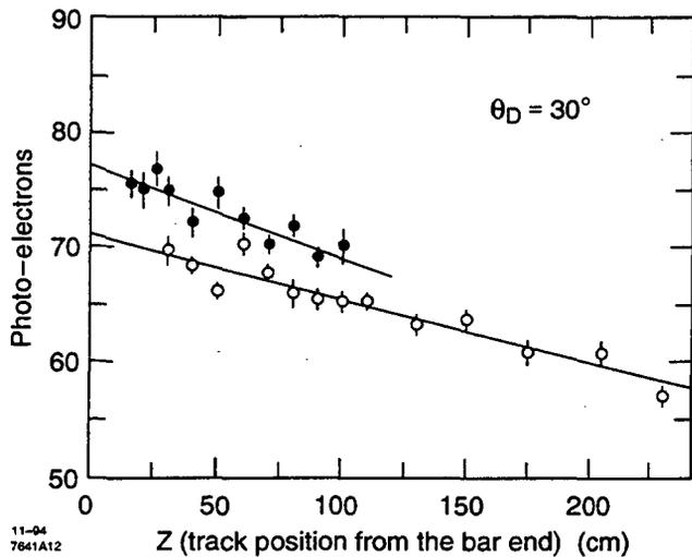
Figure 6: Track position dependence of the photo-electron yield at a dip angle  $\theta_D = 30^\circ$ . The solid circles are measurements with the 120 cm long bar and the open circles are with the 240 cm long bar. The solid lines are exponential fits to the data with an effective attenuation rate of 11.2 %/m and 8.7 %/m, respectively.
