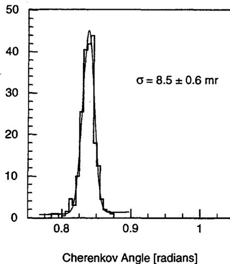
Figure 7: Single Cherenkov photon angle distribution at  $\theta_D = 30^\circ$ ,  $l=90$  cm, and  $z = 205$  cm with the 240 cm long bar. The line is a fit of a Gaussian plus polynomial to the data. The width of the fit is  $8.5 \pm 0.6$  mr.
