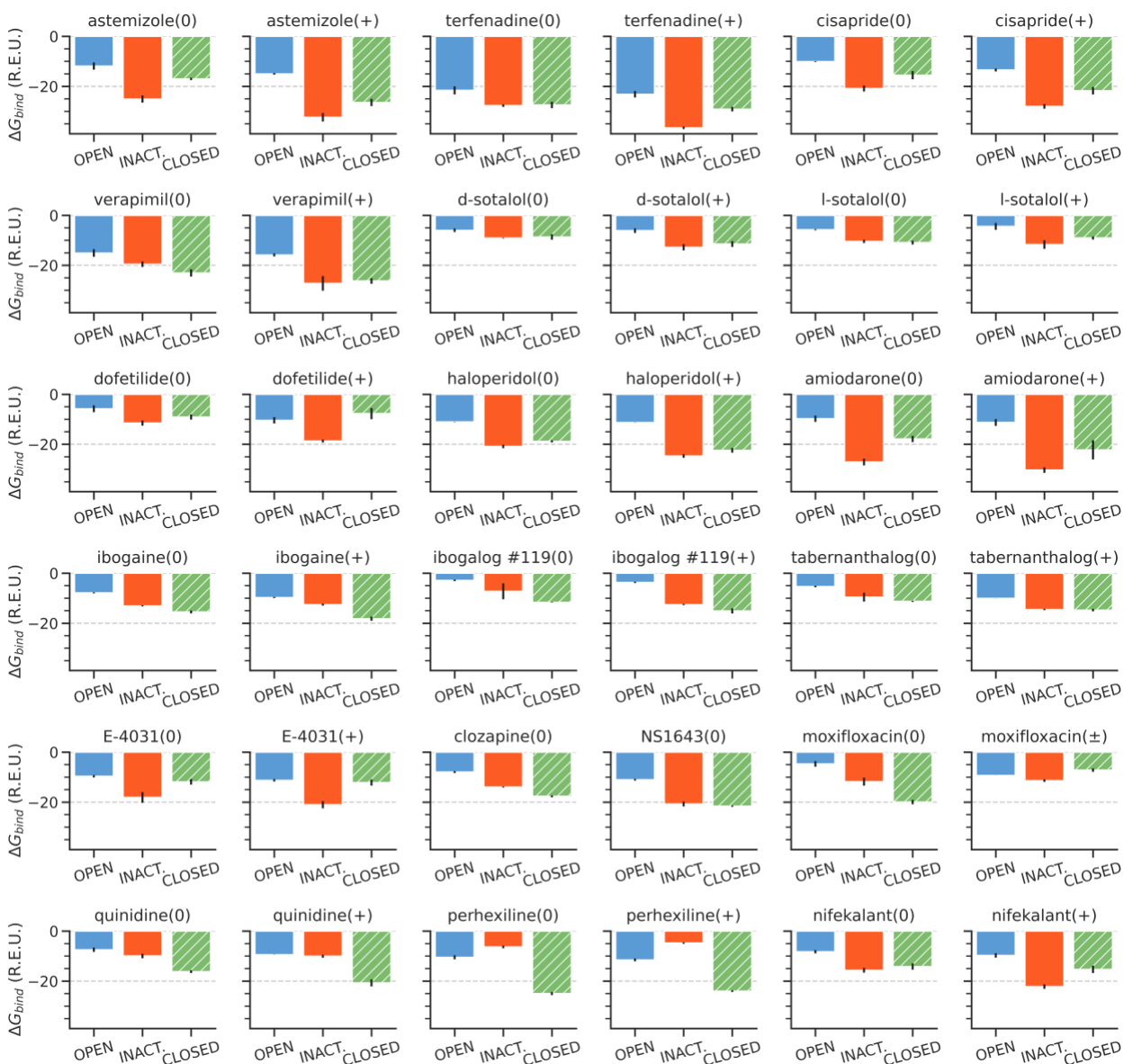
Figure 8. GALigandDock drug docking results to different hERG channel models. Each bar plot represents the estimated energy of binding in Rosetta energy units (R.E.U.) for the named drug to the open-, inactivated-, and closed-state hERG channel models. Lower values mean more favorable binding. 25,000 docking poses were generated for each drug/channel model pairing. The top 50 poses were clustered, and the plotted energy represents the average
