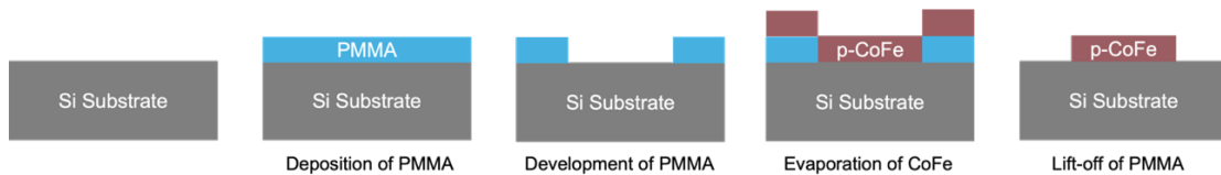
Figure 5.1. Illustration of fabrication process for poly-crystalline CoFe nanomagnet.
