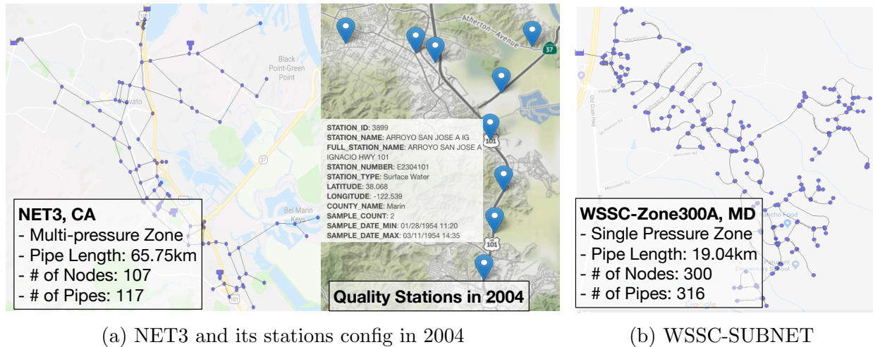
Figure 6.8: Two real-world water networks: (a) a multi-pressure zone of NMWD; (b) a single pressure zone of WSSC.
