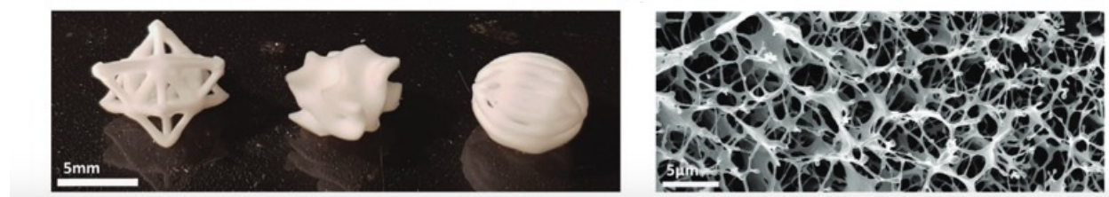
Figure 2.25 3D printed octet-truss, gyroid, and ovoid structures from a modified x_{0.4} PNIPAM precursor solution (left) and SEM of the 3D printed PNIPAM, confirming open-celled pore structure (right).
