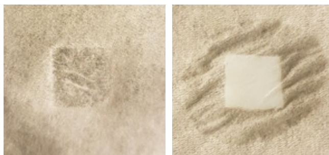
Figure 2.27 Capillary wicking of water by a tissue after 1 minute for x_{1.0} PNIPAM (left) and x_{0.4} PNIPAM (right) hydrogels.
