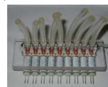
Fluidic multiplexer for calibration
