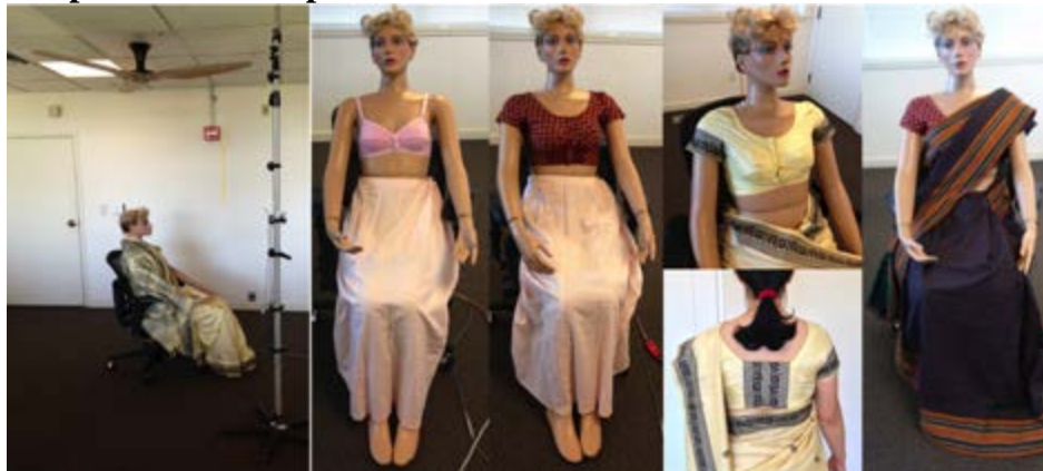
Figure 6. (Left to right) The test conditions of the climate chamber showing the data-logger setup; manikin with petticoat, panty, bra and bodice; a rear view of a sari and bodice on a human subject; manikin in a sari ensemble
