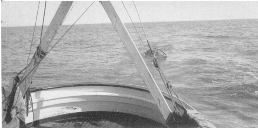
FIG. 21. The plankton net is being lowered away. As the vessel moves ahead at a set speed, the net is paid out at the rate of about 18 meters per minute so that at the completion of 14 minutes, 250 meters of wire are out. The boat is then stopped, and six minutes are required to haul the net aboard; thus a quantitative haul of 20 minutes' duration is completed. Photograph by Donald H. Fry, Jr., 1931.
