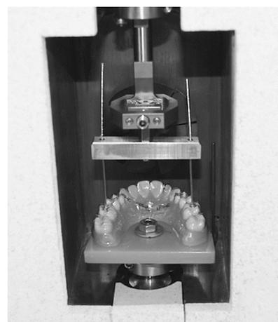
**Figure 1. Mechanical Retention Setup for Clear Aligners with Attachments.** Image borrowed with permission from Kwak *et. al.*, 2015
