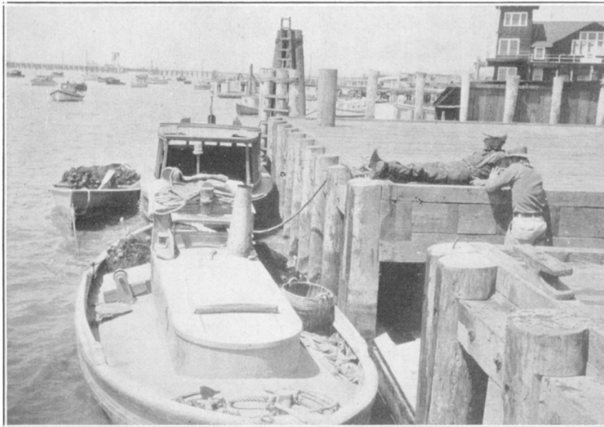
FIG. 8. A typical boat used in San Francisco and San Pablo bays for netting striped bass and other species. Note the wide beam, the house and the trailing dory. Photograph by E. C. Scofield, August, 1927.
