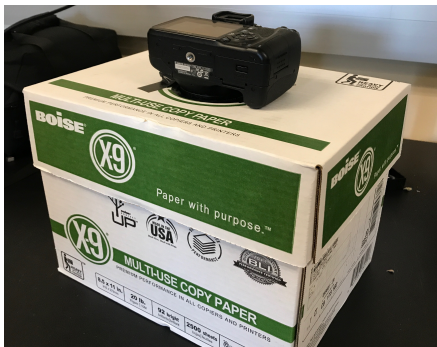
(a) Measurement enclosure to prevent external light from entering
