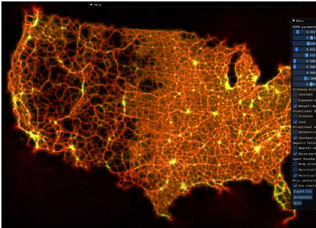
Figure 1.2: A map showing how PolyPhy’s simulated Physarum polycephalum agents would have designed the highway system of the United States of America [16].
