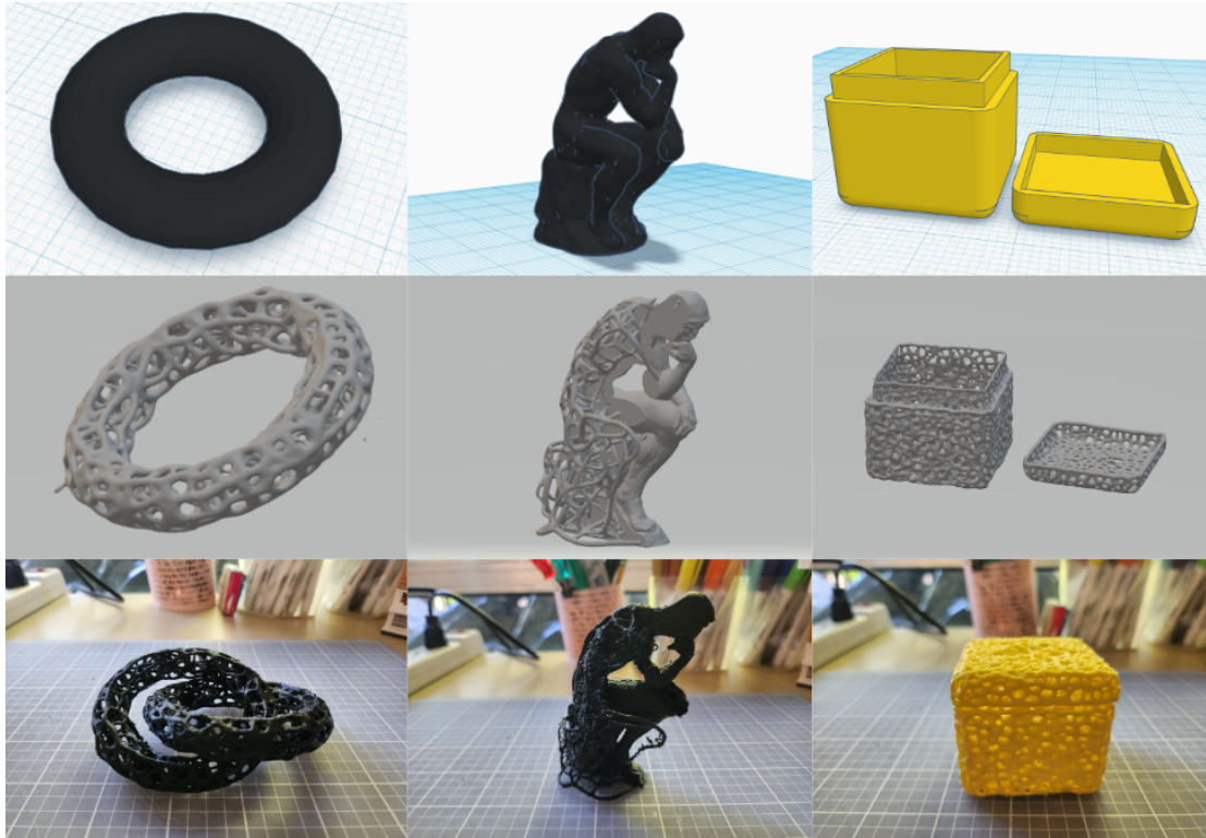
Figure 2.9: The original meshes for each shape (top row), the reconstructed mesh produced by PolyPhy (middle row), and the final printed objects (bottom row). The bottom left image is a pair of torii printed in such a way that they are linked together. The bottom middle image is of "The Thinker" by Rodin except that half of the model has been replaced with the result of the model being passed through PolyPhy. The bottom right image is a simple box and lid.
