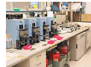
Equipment layout for final manual Fosmid processing steps: ethanol drying, resuspension, incubation, and reformatting into 384-well plates.
