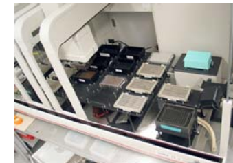
The Biomek FX Workstation used for the first half of the Fosmid processing
