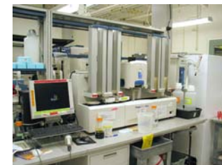
The Platemate Plus Automated Pipettor used for inoculating into 96-well plates from 384-well plates
