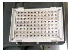
The LBNL custom 96-well magnet has superior magnetic holding strength and draws beads into a ring pattern at the bottom of well
