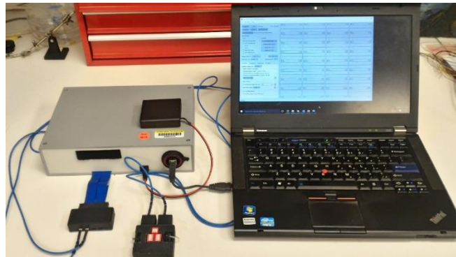
Figure 2-3: Ephys system connected and running using a modified version of the Intan’s compiled software. The power isolator and RHD 2000 Board are housed in grey enclosure. Two RHD2164 headstages are connected to the system to the electrode adapter housed in 3D printed cases.
