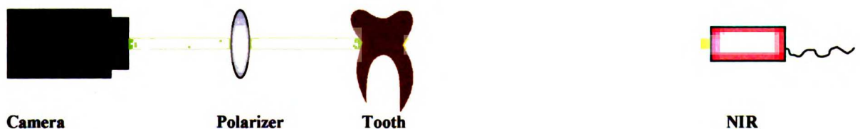
Figure 4 NIR Transillumination setup for buccal lesions. The NIR light comes behind the tooth and travels through cross polarizers before reaching and illuminating the tooth. The InGaAs focal plane array is in front of the tooth and takes an image of the buccal surface of the tooth.
