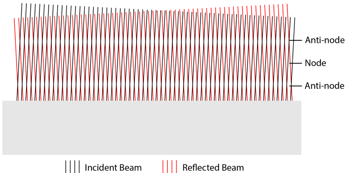
Figure 2.8. Interference of incident and reflected x-ray beams, leading to regions of high and low electric field intensity.
