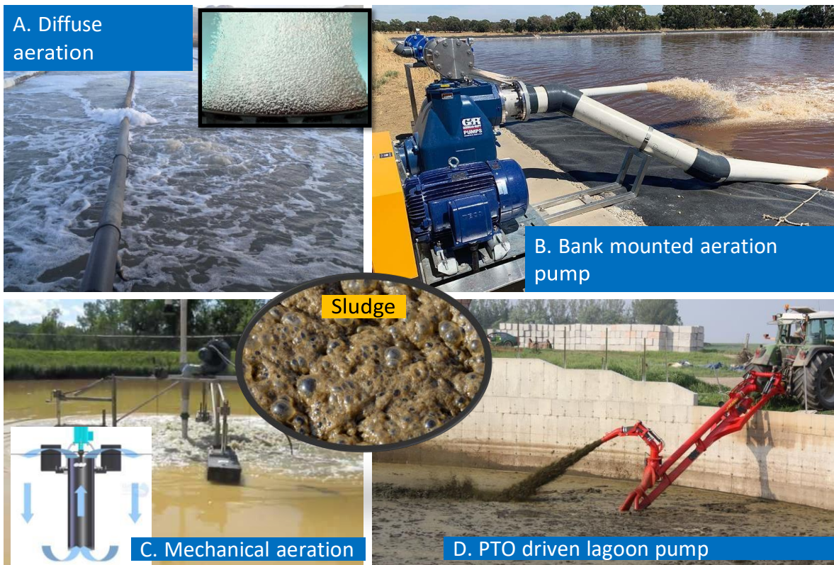
Figure 1.1: Aeration of dairy manure slurry: A) diffuse aeration; B) aeration by bank mounted aeration pump; C) mechanical aeration; and D) tractor PTO driven lagoon pump. Modified online images [A, B, C, D]. Available from: https://blog.wastewater.com/technical-bulletin-178-selecting-lagoon-aeration-systems/ ; https://www.netsolwater.com/mechanical-wastewater-vs-diffused-air-aeration-systems.php?blog=2007 ; https://www.hydroinnovations.com.au/training/aeration-systems-are-important ; http://nuhn.ca/products/manure-pumps/lagoon-pump/ ; https://www.youtube.com/watch?v=YctXi9jDK8U . [Accessed 3 December, 2023].
