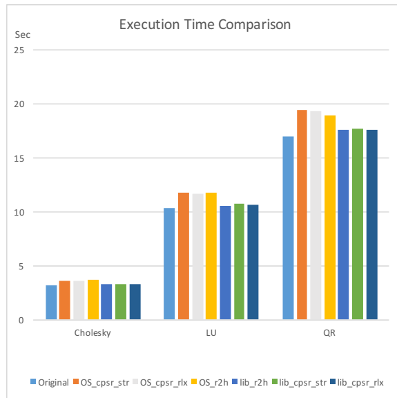
Figure 4.7: Execution time of Cholesky, LU and QR factorization using several different energy saving solutions. Right two bars in each group show our results, which have similar performance than existing state-of-the-art solutions.
