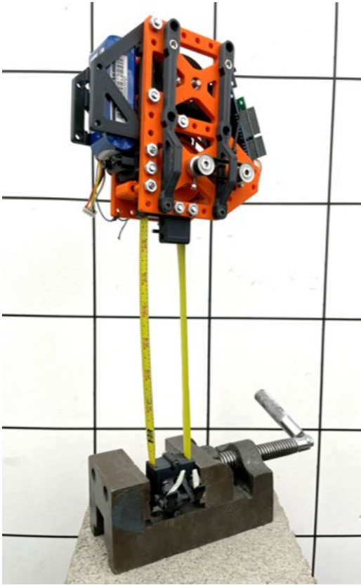
Fig. 10: EEMMMa-1 standing demonstration. The limb is deployed downward, with the end effector secured in a vice. The weight of the main body loads the limb in compression, similar to a weight-bearing leg.
