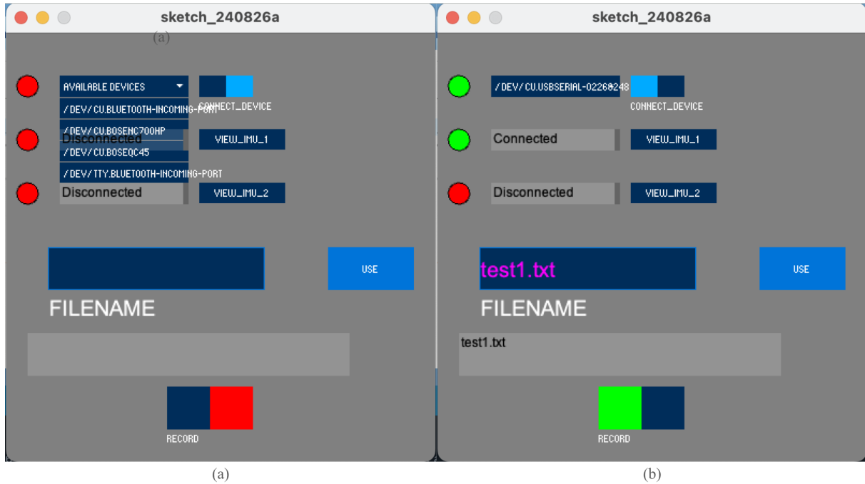
Figure 5.3. Data acquisition interface using the Processing 4 software, (a) The interface gives you an option of boards to select from, (b) When connected, the status of the corresponding boards turn green; can record the data in a file named by your choice.
