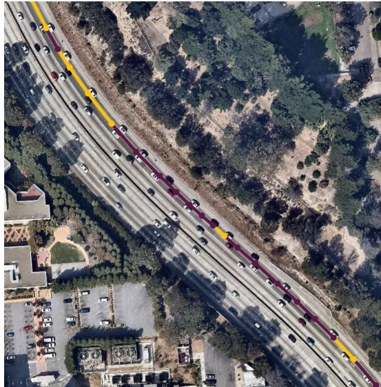
Figure 4.4: Naive assignment resulting in excessive lane changes
