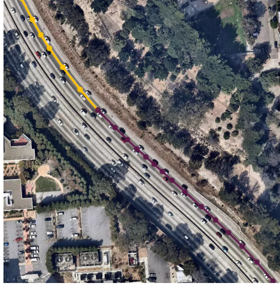
Figure 4.8: Viterbi lane assignment of trajectory shown in figure 4.4.
