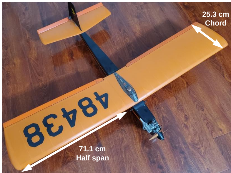
Figure 5.9: Remote controlled model aircraft used for this study and its half span and wing chord dimensions. This aircraft is the Carl Goldberg Falcon Mark II Remote Controlled Aircraft.
