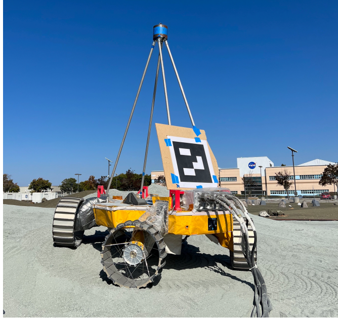
Figure 2.8: MGRU-CG performing a point turn on a 10^\circ slope in the Roverscape. ArUco markers were used for motion capture.
