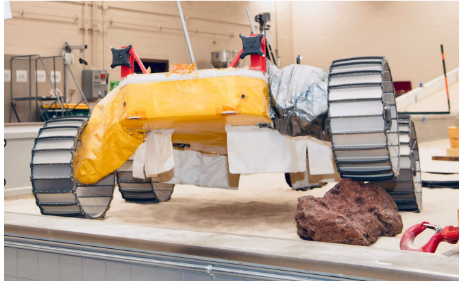
Figure 2.7: MGRU’s actuated suspension. Each wheel module has suspension, steering, and propulsion motors. Actuation of the suspension allows MGRU to keep its wheels on the ground when one wheel climbs a rock.
