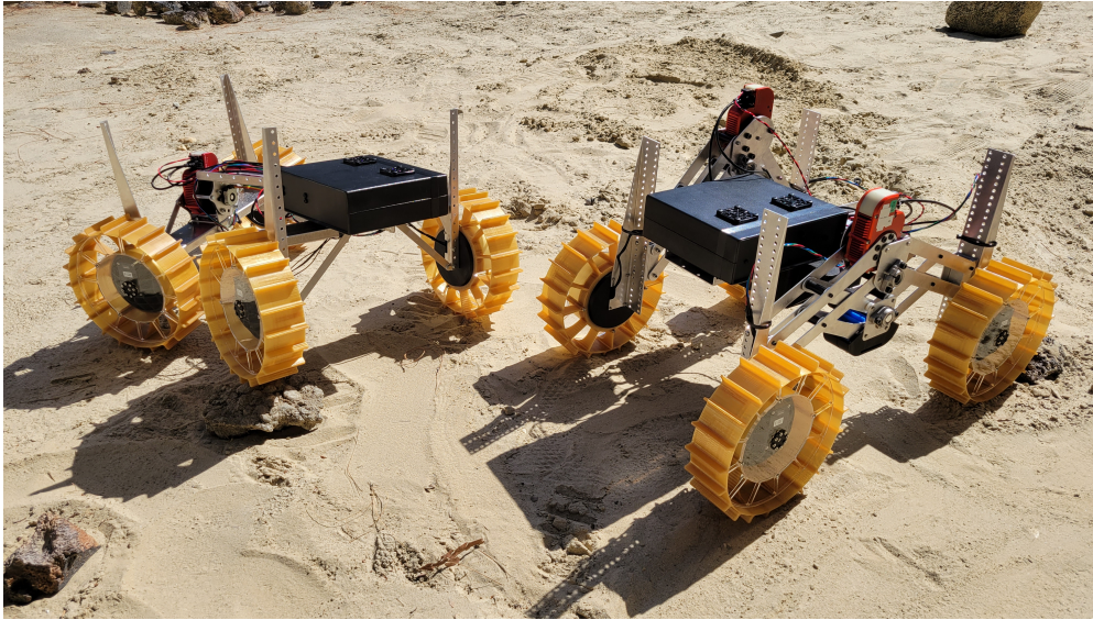
Figure 3.26: Asterix and Obelix. These rovers can collectively perform five articulated locomotion gaits, some of which can actively modify load distribution. They have the same vehicle parameters, and their kinematics and center of mass can be adjusted to test other metrics of interest.
