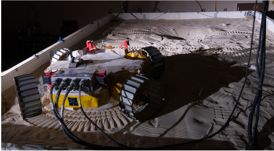
Figure 1.3: Mobility validation testing at NASA Glenn Research Center’s SLOPE Lab. The rover is commanded to traverse a scene covered in rocks and craters that are estimated to be representative of the lunar surface.
