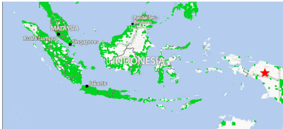
Figure 3.3: Indonesian cellular coverage as of 2013 across all carriers. Wide swaths of sparsely populated parts of the country lack any cellular coverage, which includes at least 10 million people. The red star on the right marks the location of the Papua CCN.
