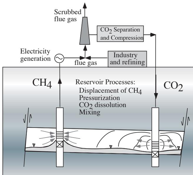
**Figure 1.** Schematic of CSEGR processes.
