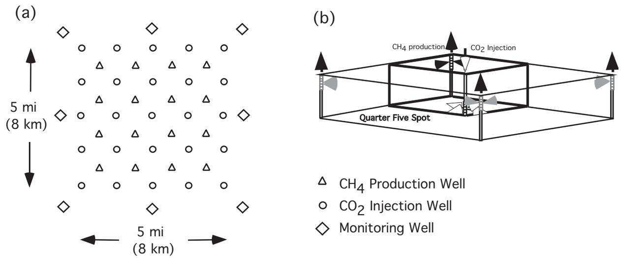
**Figure 2.** (a) Schematic of well pattern for CSEGR with well spacing of one mile (1.61 km). (b) Perspective view of quarter five-spot simulation domain.
