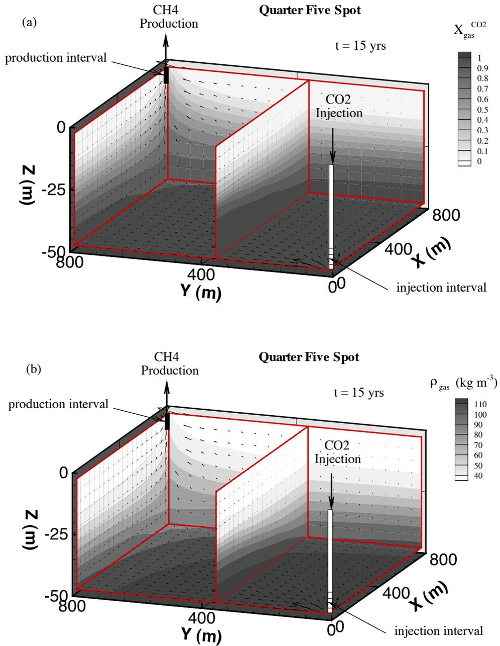
**Figure 3.** (a) CO<sub>2</sub> mass fraction in the gas and (b) gas density after 15 years of injection into the lower part of the reservoir.
