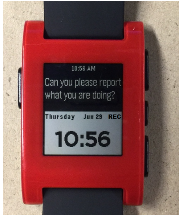
Figure 4.4: Watch — open-ended notification. This is only useful as a reminder; to initiate reporting labels the user has to go to the phone. During a 20-second recording window, the text “REC” is shown in the bottom half.
