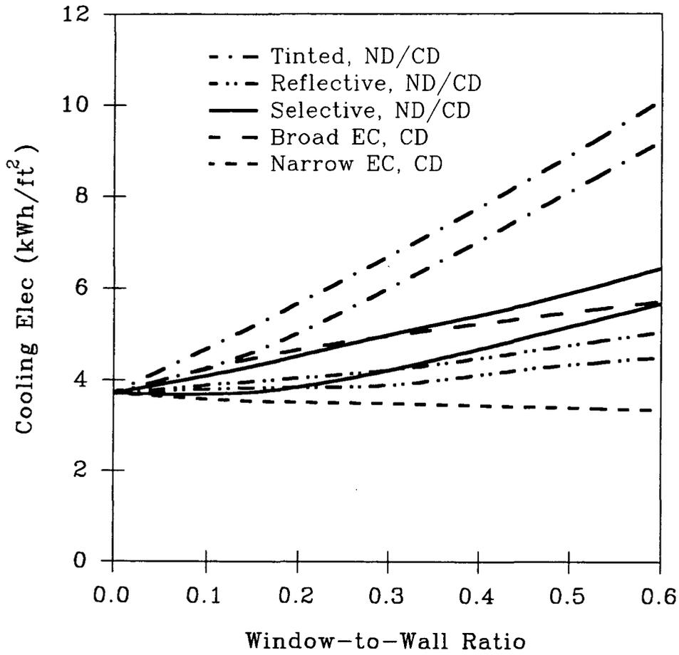
Figure 4. Annual Cooling Electricity Consumption for the Five Window Prototypes in the West Perimeter Zone
