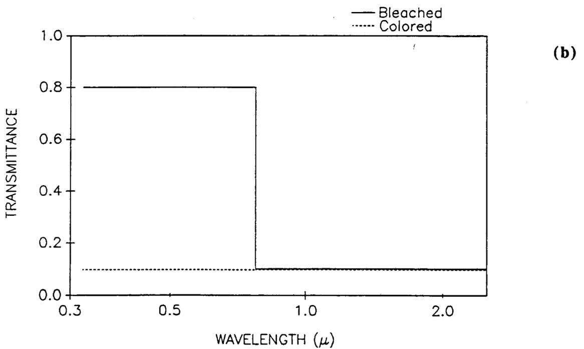
Figure 1. Solar Transmittance Spectra of the (a) Broad-band Electrochromic and (b) Narrow-band Electrochromic Glazing Prototypes
