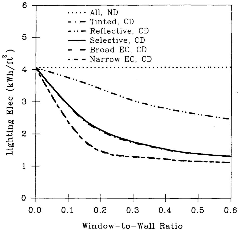
Figure 3. Annual Lighting Electricity Consumption for the Five Window Prototypes in the West Perimeter Zone
