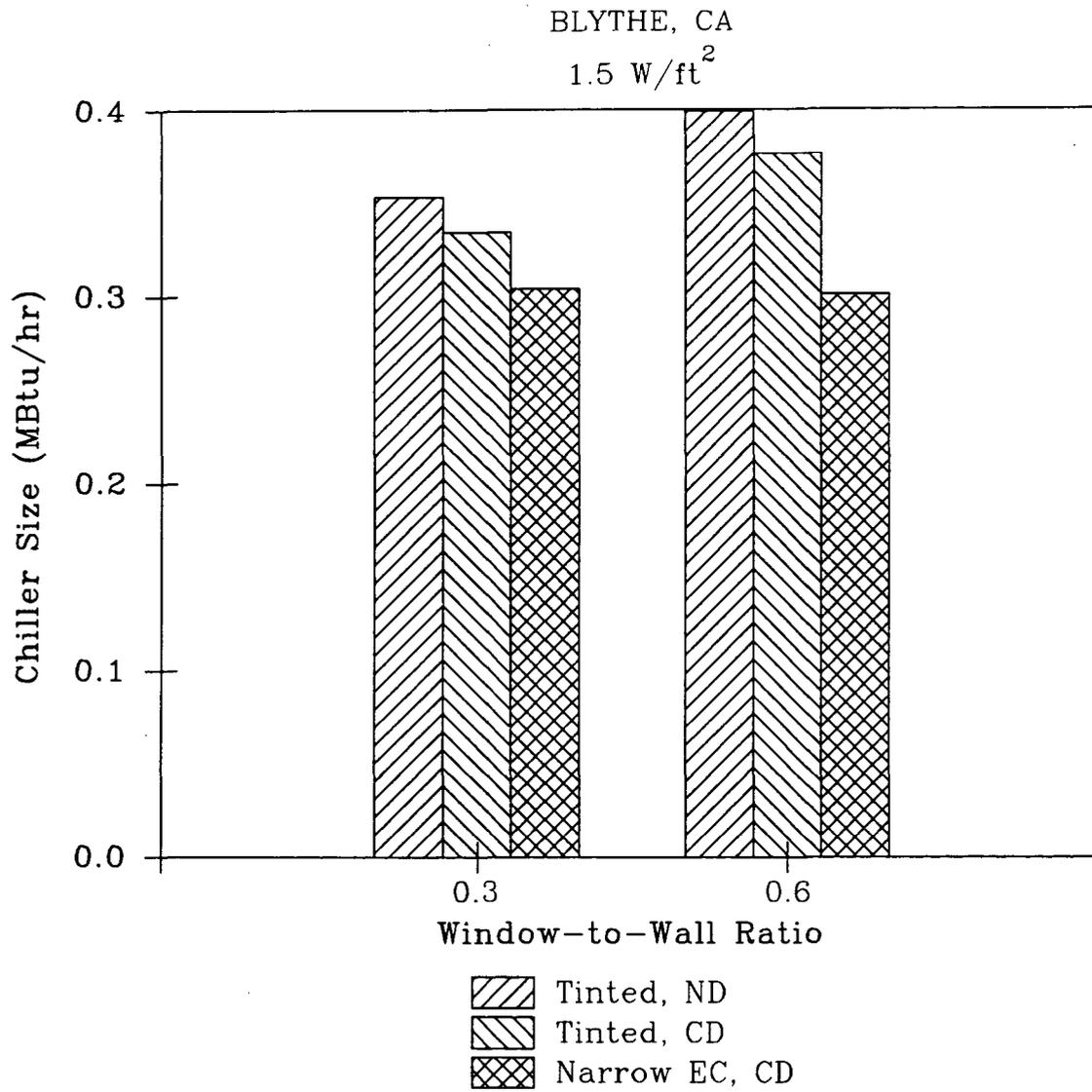
Figure 8. Total Perimeter Zone Chiller Sizing for Selected Window Prototypes
