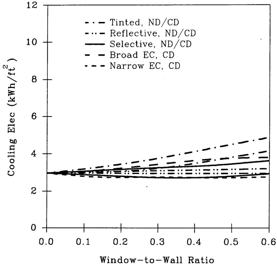
Figure 5. Annual Cooling Electricity Consumption for the Five Window Prototypes in the North Perimeter Zone
