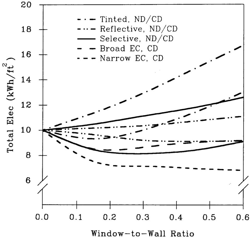
Figure 6. Total Perimeter Zone Annual Electricity Consumption for the Five Window Prototypes
