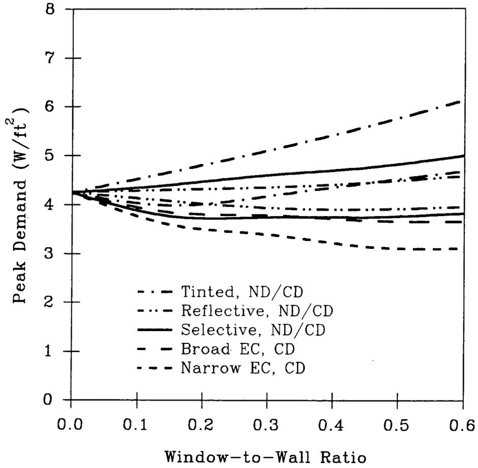
Figure 7. Total Perimeter Zone Peak Electricity Demand for the Five Window Prototypes
