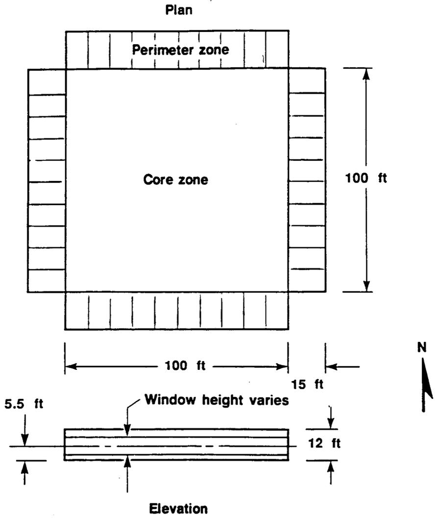
Figure 2. Office Building Module Used in the DOE-2 Building Energy Simulations
