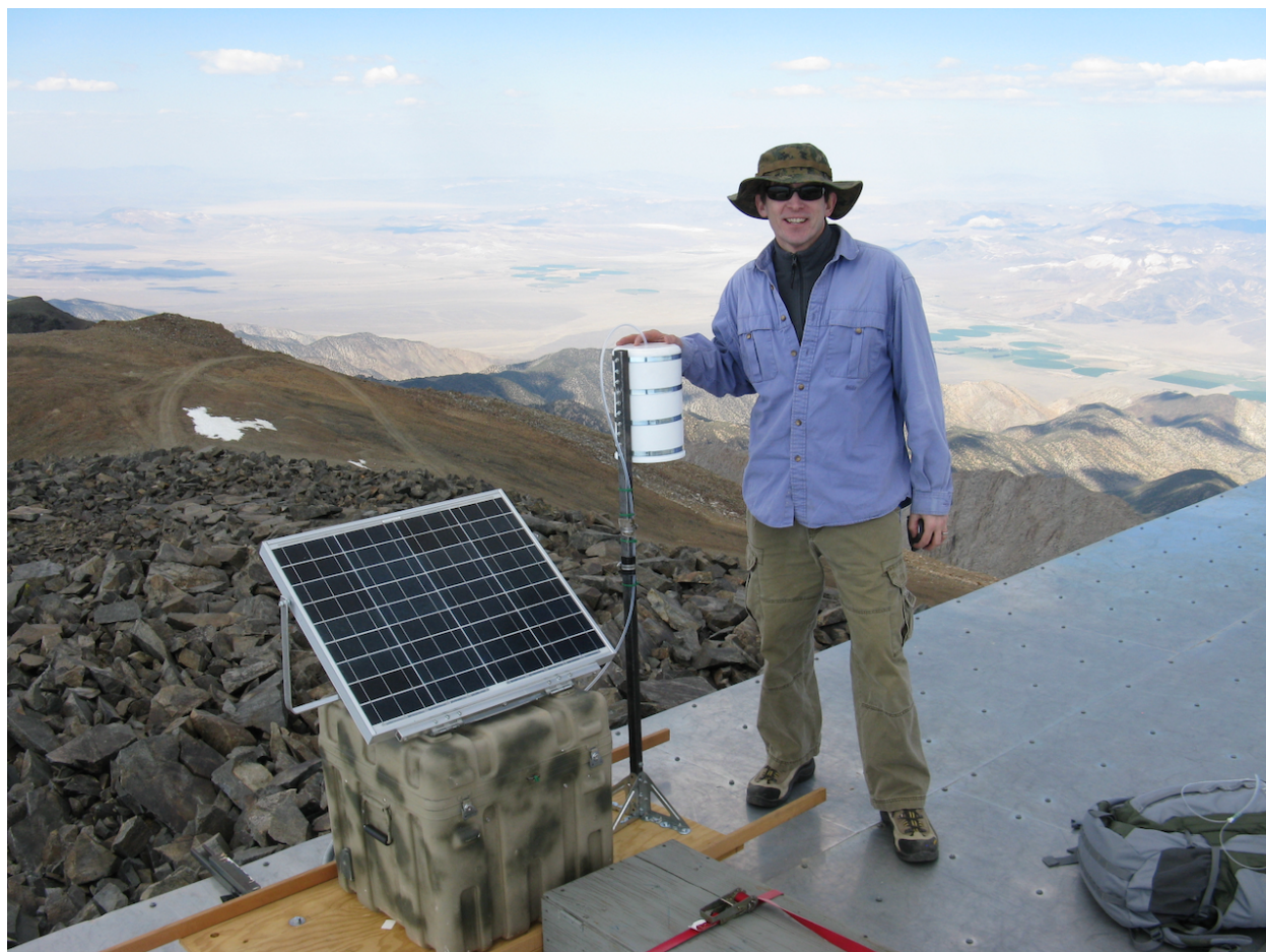
Fig. 3. Joel Burley with the initial installation of the Summit Hut ozone experiment, in August of 2009. The sampling inlet is protected by the inverted Teflon beaker, which acts as a rain shield. The camouflage-painted shipping case contains the 2B ozone monitor, a 12-volt battery, and a solar charge controller.
