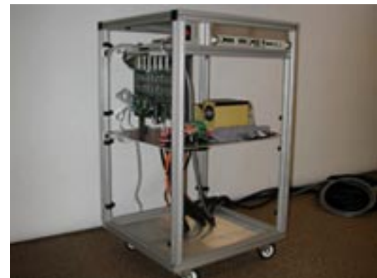
Fig. 5. (a) A photograph of the actual PEM gantry which is fully loaded with the complete data acquisition electronics (but not loaded with detector modules). Each detector bank utilizes nine (side bank) or twelve (top/bottom bank) detector modules. The detector modules are loaded into a can (Fig 4) with the Kapton "flex tail" feeding out between the detector modules and connecting to the readout electronics. (b) PEM camera electronics cabinet. There is space for the computer on the bottom. The Coincidence Processor and power supplies are visible in the middle area, and the HV power panel is seen on the top.
