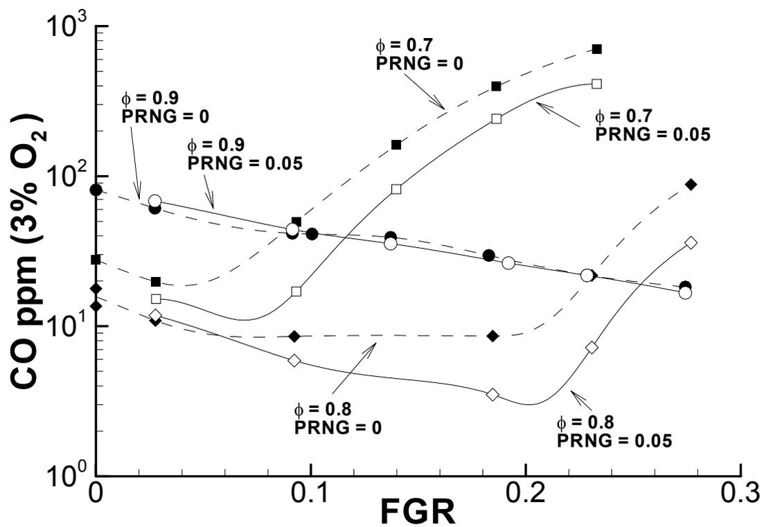
Figure 6. NO<sub>x</sub> and CO emissions as functions of  $\phi$ , external FGR and PRNG from a catalytic reformer.
