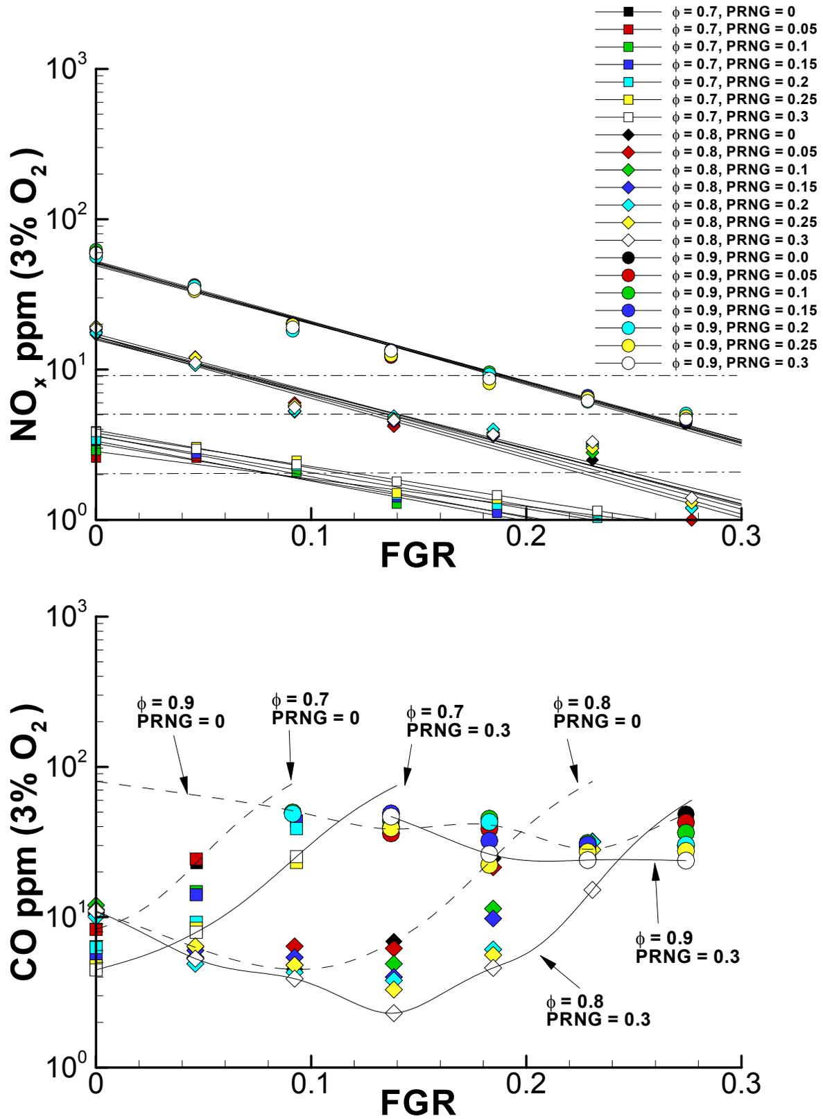
Figure 3.  $\text{NO}_x$  and CO emissions as functions of  $\phi$  and simulated FGR and PRNG.
