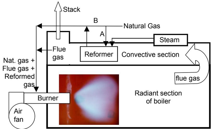
Figure 1. Adaptation of FGR/PRNG concept to packaged boiler of 300 KW to 8 MW. Picture shows a 0.6 kW flame generated by a  $R_b = 3.8$  cm LSB.
