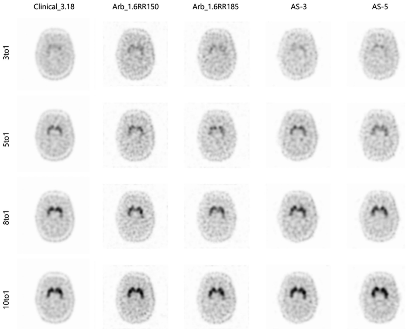
FIG. 9. Reconstructed images with 150 iterations and CDR correction for I-123 brain DaT imaging from the three configurations of the conventional scanner and our proposed scanner in AS-3 and AS-5 acquisition modes as a function of striatal-to-background activity ratio. All images in each row were normalized by the maximum value in the images for 10–1 striatal/background ratio and postprocessed using a 3D Gaussian filter with a sigma of 1 pixel.
