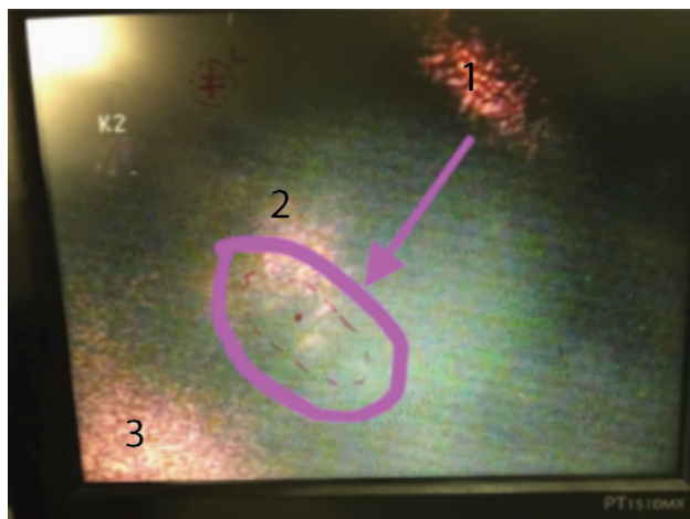
Figure 3.14: Topmost reflection (#1, rock surface) must be placed into the focal point of the beam (circled in pink) which is determined by the beamline scientist at the start of every accelerator run cycle. Reflections #2 and #3 are from the top and bottom of the glass slide.
